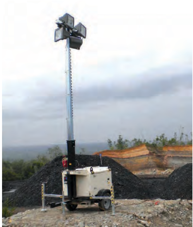
1 Linktower 4x400W MH can be connected to the extra outlet of a VT8 (3KVA)
